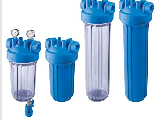
The new range of DP BIG housings is designed to fit to "BIG" filter cartridges with outer diameter (OD) from 4" to 4.50", inner diameter (ID) 1.10", height at 10" and 20" with standard SX (DOE) configuration. With female IN/OUT connections at 1" and 1"1/2, with BSP or NPT plastic threads DP BIG housings are suitable for every domestic Point-of-Entry (POE) or every industrial application when heavy-duty performance is a must.
