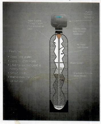
The formation of oxygen into ozone occurs with the use of energy. In general, an ozone water treatment system includes passing
